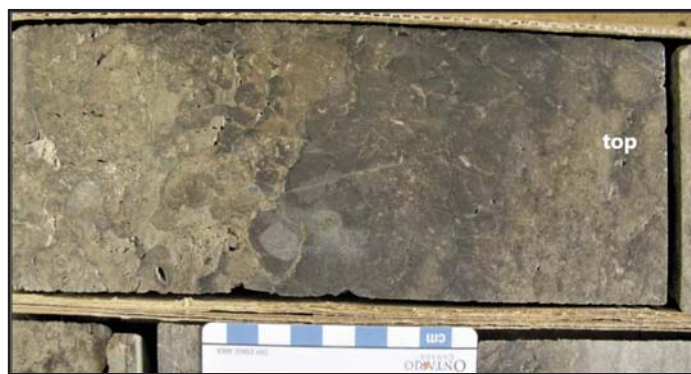
Figure 22. Dark brown to black, dolostone paleokarst rubble in the inter-pinnacle Guelph Formation, 800.5 m below rig floor. Drill core from petroleum well Tec. Dow 4, Moore 21-XII, in Lambton County, well licence #T007290, core # 996 at the OGSRL. This paleokarst rubble forms a regional brine aquifer in the regional karst and inter-pinnacle karst belts in southern Ontario.
