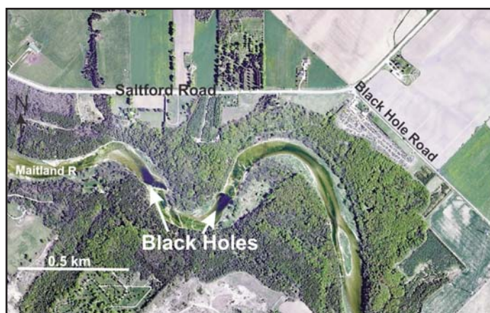
Figure 15. Aerial photograph of the Maitland River west of Goderich showing "black holes" in bed of Maitland River marking location of submerged sinkholes that are over 10 m deep in the Dundee and Lucas formations. The sinkholes provide entry points for infiltration of meteoric water into the bedrock.
