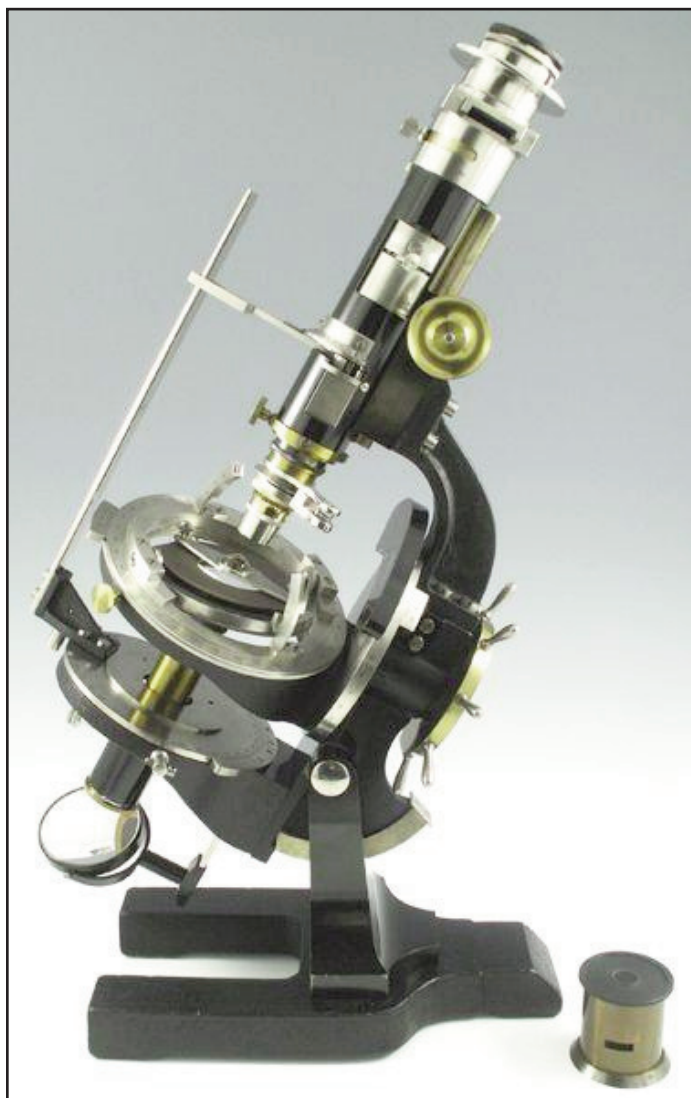
Figure 1. Petrographic microscope with a universal stage (Kile 2009).
